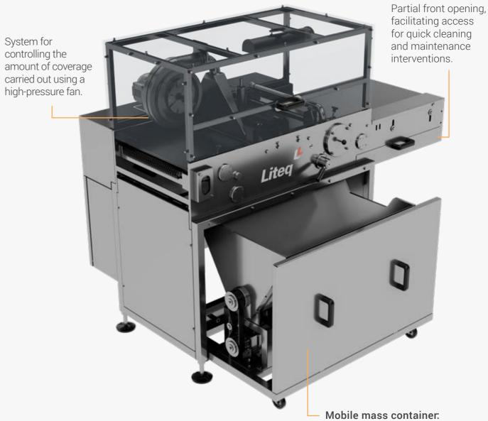
facilitates setup and cleaning, jacketed and with special stirrer, equipped with positive recirculation pump.
